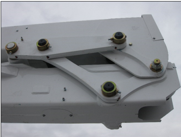
All Fasteners and pins in place
