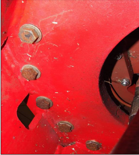
Turtable bearing bolts in place and torqued, Pedestal to bearing and turtable to bearing
