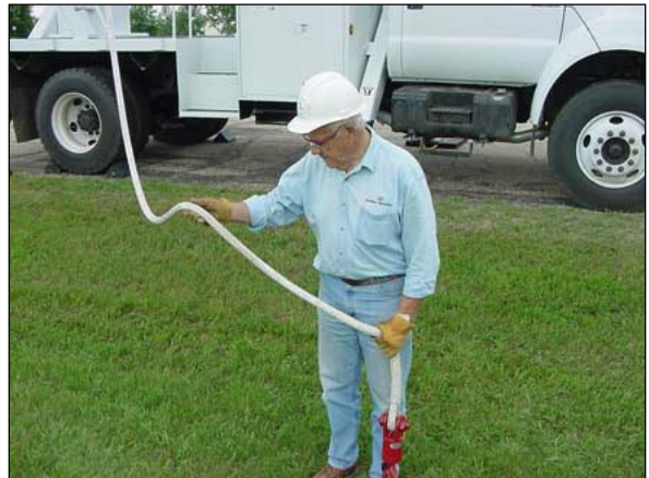
Inspect all load lines and lifting rigging
