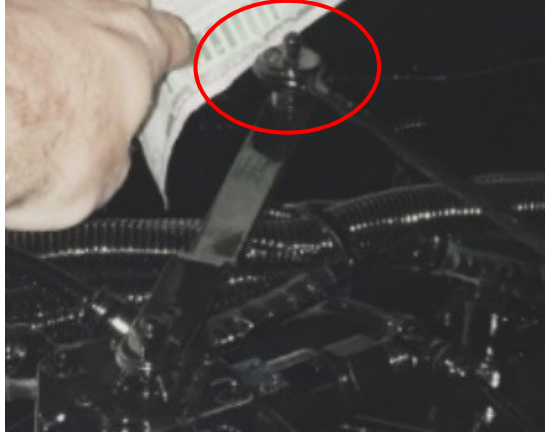
Figure 2. Top end of ride height control linkage
